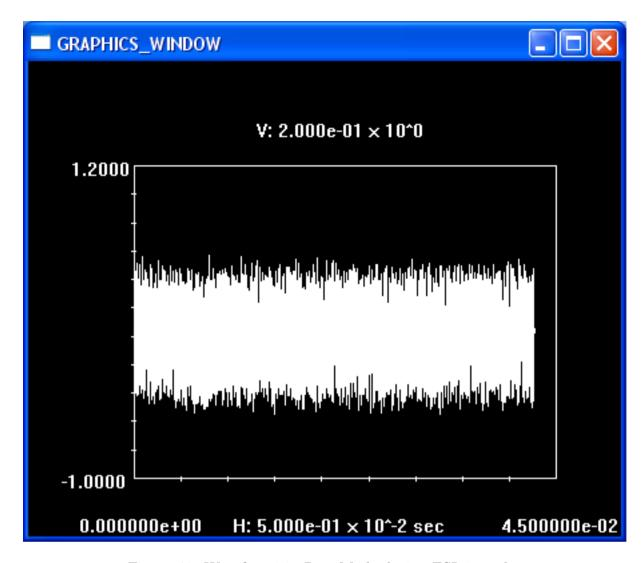
Figure 40: Waveform1 in Raw Mode during ESL impedance measurement.
