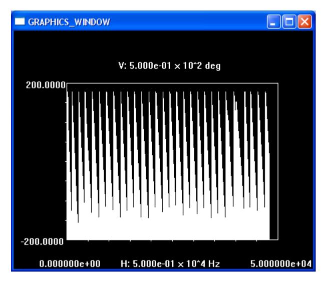
Figure 18: Phase response of Fig. 12 obtained using the H option.
