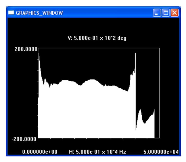
Figure 19: Phase response in Fig. 18 after removing 0.6ms delay using the G option.
