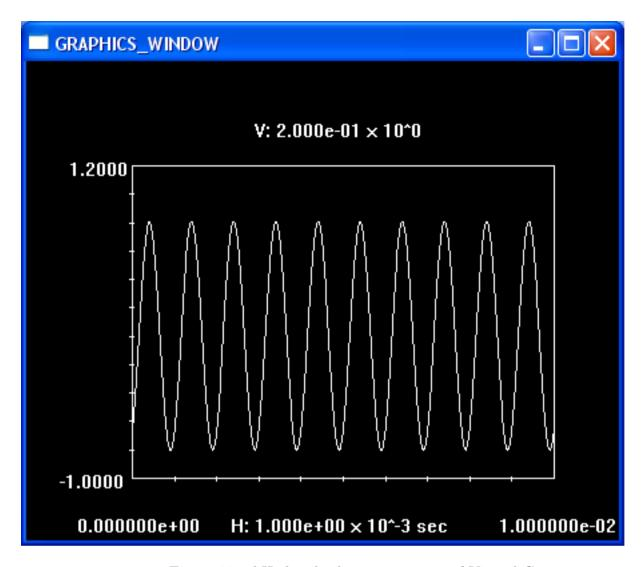
Figure 38: 1kHz loopback sine wave test of Virtual Crossover.
