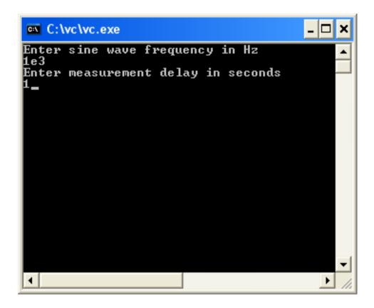
Figure 23: Setting up a 1kHz sine wave using the S option.
