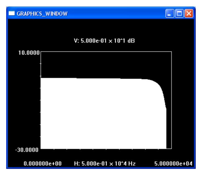
Figure 37: Frequency response of Virtual Crossover loopback from MLS measurement.
