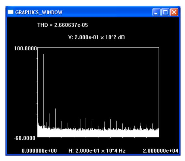
Figure 39: Frequency response magnitude and THD+N of 1kHz sine wave loopback test.
