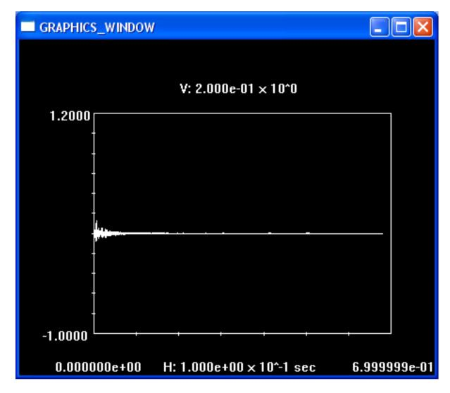
Figure 8: Measured impulse response of Vifa D26TG-35 tweeter.
