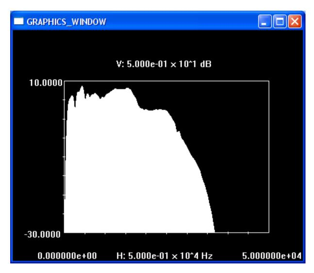
Figure 15: Magnitude of the frequency response of the waveform in Fig. 12.
