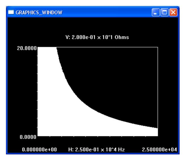
Figure 43: Input impedance magnitude of electrostatic panel.
