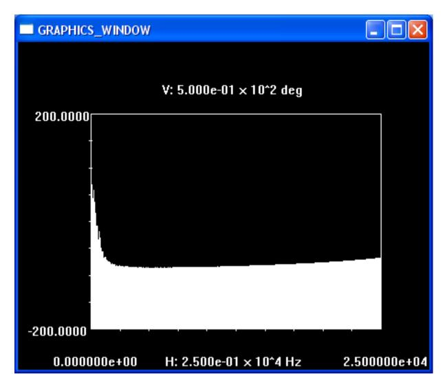
Figure 44: Phase angle of electrostatic panel input impedance.
