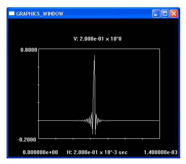
Figure 36: Impulse response of Virtual Crossover loopback from MLS measurement.
