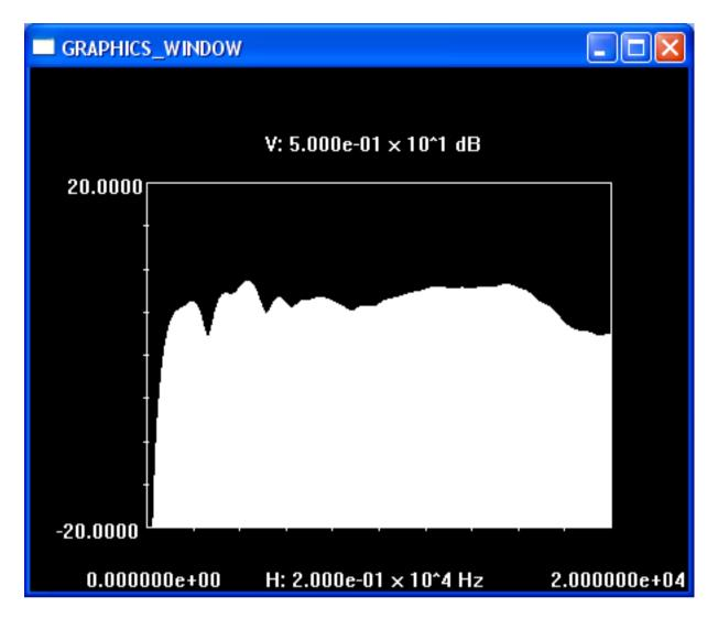
Figure 17: Frequency response of Fig. 12 with adjusted vertical axis limits, using the P option.
