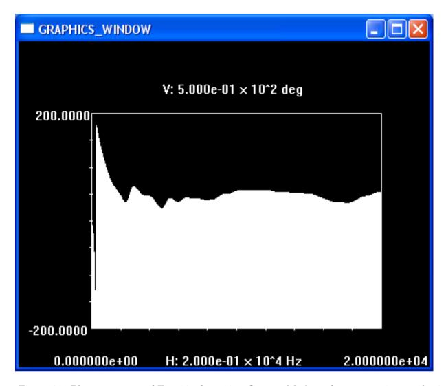
Figure 20: Phase response of Fig. 19 after using Cursors Mode to focus attention on the 0-20kHz range.
