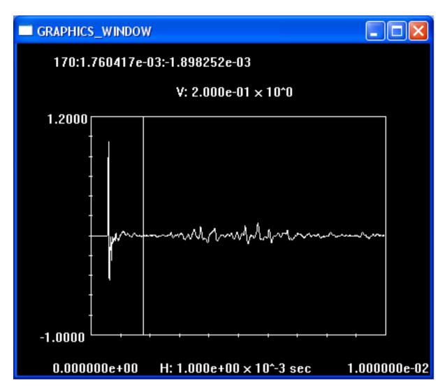
Figure 11: Plot of Fig. 10 in Truncation mode with vertical line at one possible truncation point between primary tweeter response and room reflections.
