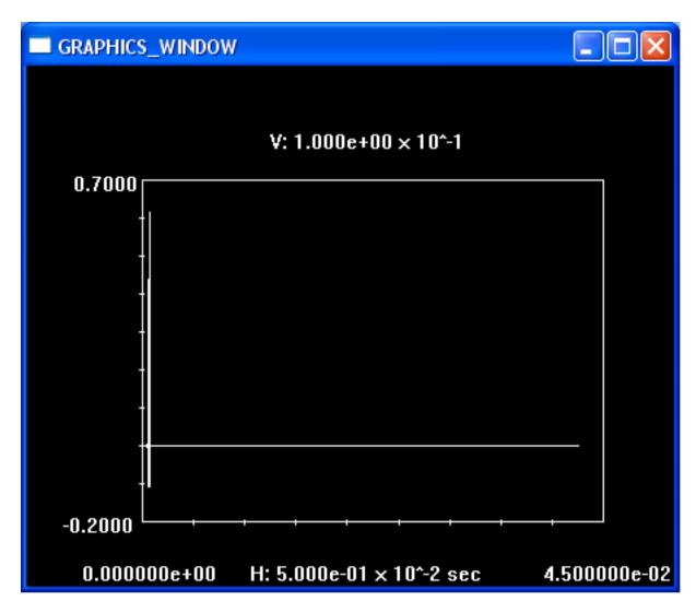
Figure 41: Impulse response of waveform 1 during ESL impedance measurement.
